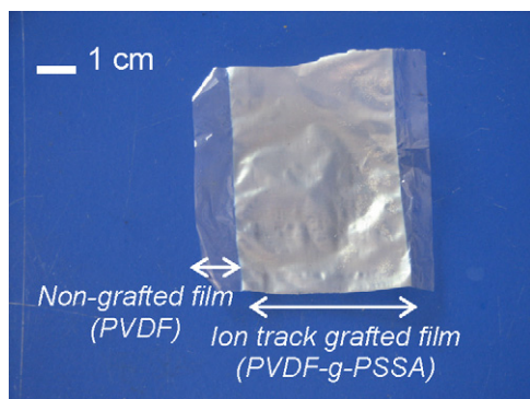
Fig. 2. Photograph of an ion track grafted PVDF-g-PSSA membrane (fluence 10^{10} \text{ cm}^{-2} ): white part corresponds to the radiografted part (grafting yield of 140 wt%), translucent part corresponds to the non-irradiated part (SHI beam width = 4 cm).
